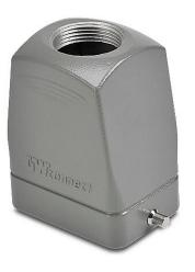
ZIPport hood housing, 2-peg, top entry, connector housing size 6B, (1) Pg 21 threaded hole, high construction, heavy-duty die cast aluminum. For use with ZIPport size 6B single lever connector housings.
