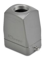
ZIPport hood housing, 2-peg, top entry, connector housing size 6B, (1) Pg 21 threaded hole, high construction, heavy-duty die cast aluminum. For use with ZIPport size 6B single lever connector housings.
