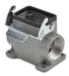
ZIPport surface mount housing, single lever, connector housing size 6B, (2) Pg 29 threaded holes, high construction, heavy-duty die cast aluminum. For use with ZIPport size 6B 2-peg connector housings.
