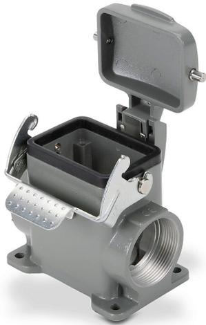
ZIPport surface mount housing, single lever, standard, connector housing size 6B, (2) Pg 29 threaded holes, high construction, heavy-duty die cast aluminum. For use with ZIPport size 6B 2-peg connector housings.
