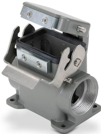
ZIPport surface mount housing, single lever, automatic closing, connector housing size 6B, (2) Pg 29 threaded holes, heavy-duty die cast aluminum. For use with ZIPport size 6B 2-peg connector housings.
