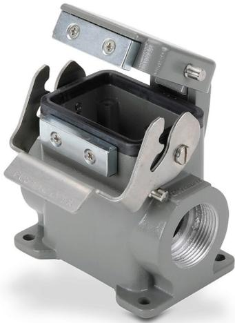
ZIPport surface mount housing, single lever, automatic closing, connector housing size 6B, (2) Pg 21 threaded holes, heavy-duty die cast aluminum. For use with ZIPport size 6B 2-peg connector housings.
