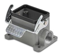
ZIPport surface mount housing, single lever, connector housing size 6B, (2) Pg 16 threaded holes, heavy-duty die cast aluminum. For use with ZIPport size 6B 2-peg connector housings.
