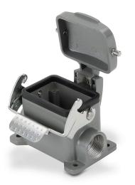
ZIPport surface mount housing, single lever, standard, connector housing size 6B, (2) Pg 16 threaded holes, heavy-duty die cast aluminum. For use with ZIPport size 6B 2-peg connector housings.
