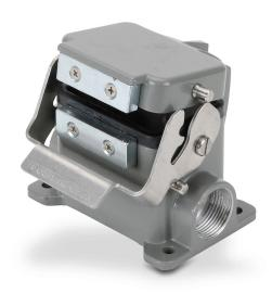
ZIPport surface mount housing, single lever, automatic closing, connector housing size 6B, (2) Pg 16 threaded holes, heavy-duty die cast aluminum. For use with ZIPport size 6B 2-peg connector housings.
