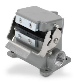
ZIPport surface mount housing, single lever, automatic closing, connector housing size 6B, (2) Pg 16 threaded holes, heavy-duty die cast aluminum. For use with ZIPport size 6B 2-peg connector housings.
