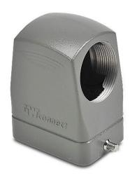
ZIPport hood housing, 2-peg, side entry, connector housing size 6B, (1) Pg 29 threaded hole, high construction, heavy-duty die cast aluminum. For use with ZIPport size 6B single lever connector housings.
