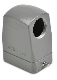
ZIPport hood housing, 2-peg, side entry, connector housing size 6B, (1) Pg 21 threaded hole, high construction, heavy-duty die cast aluminum. For use with ZIPport size 6B single lever connector housings.
