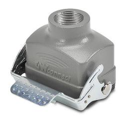
ZIPport coupler housing, single lever, connector housing size 6B, (1) Pg 16 threaded hole, heavy-duty die cast aluminum. For use with ZIPport size 6B 2-peg connector housings.
