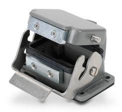
ZIPport bulkhead housing, single lever, automatic closing, connector housing size 6B, heavy-duty die cast aluminum. For use with ZIPport size 6B 2-peg connector housings.
