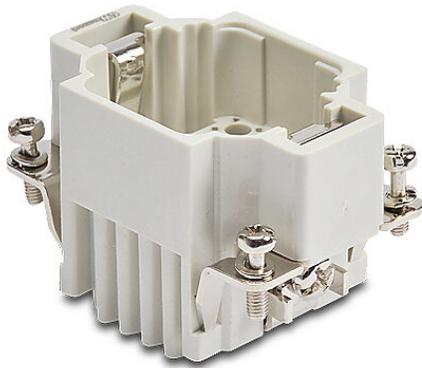
ZIPport male insert, connector housing size 6B, 24-pole, crimped contact, 10 amp, 600 VAC/VDC, poles numbered 1 to 24. For use with ZIPport multi-wire housings. Requires 10 amp male contacts ZP-MC-CC-M10A-xxx.
