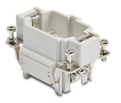
ZIPport male insert, connector housing size 6B, 6-pole, crimped contact, 16 amp, 600 VAC/VDC, poles numbered 1 to 6. For use with ZIPport multi-wire housings. Requires 16 amp male contacts ZP-MC-CC-M16A-xxx.
