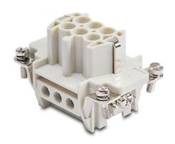
ZIPport female insert, connector housing size 6B, 6-pole, screw terminals, accepts wire size 20-14 AWG, 16 amp, 600 VAC/VDC, poles numbered 1 to 6. For use with ZIPport multi-wire housings.
