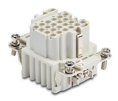
ZIPport female insert, connector housing size 6B, 24-pole, crimped contact, 10 amp, 600 VAC/VDC, poles numbered 1 to 24. For use with ZIPport multi-wire housings. Requires 10 amp female contacts ZP-MC-CC-F10A-xxx.
