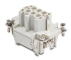
ZIPport female insert, connector housing size 6B, 6-pole, crimped contact, 16 amp, 600 VAC/VDC, poles numbered 1 to 6. For use with ZIPport multi-wire housings. Requires 16 amp female contacts ZP-MC-CC-F16A-xxx.
