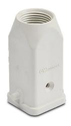
ZIPport hood housing, 2-peg, top entry, connector housing size 3A, (1) Pg 11 threaded hole, heavy-duty thermoplastic. For use with ZIPport size 3A single lever connector housings.
