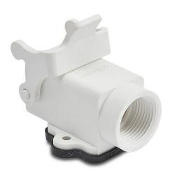
ZIPport surface mount housing, single lever, connector housing size 3A, (1) Pg 11 threaded hole, heavy-duty thermoplastic. For use with ZIPport size 3A 2-peg connector housings.
