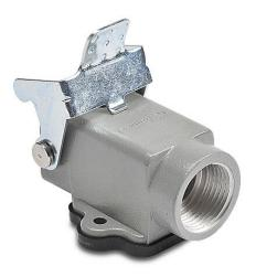
ZIPport surface mount housing, single lever, connector housing size 3A, (1) Pg 11 threaded hole, heavy-duty die cast aluminum. For use with ZIPport size 3A 2-peg connector housings.
