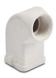
ZIPport hood housing, 2-peg, side entry, connector housing size 3A, (1) Pg 11 threaded hole, heavy-duty thermoplastic. For use with ZIPport size 3A single lever connector housings.
