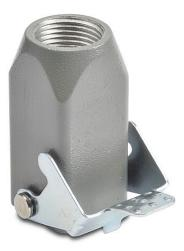
ZIPport coupler housing, single lever, connector housing size 3A, (1) Pg 11 threaded hole, heavy-duty die cast aluminum. For use with ZIPport size 3A 2-peg connector housings.
