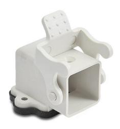
ZIPport right angled bulkhead housing, single lever, connector housing size 3A, heavy-duty thermoplastic. For use with ZIPport size 3A 2-peg connector housings.
