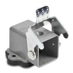
ZIPport right angled bulkhead housing, single lever, connector housing size 3A, heavy-duty die cast aluminum. For use with ZIPport size 3A 2-peg connector housings.
