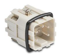
ZIPport male insert, connector housing size 3A, 4-pole, screw terminals, accepts wire size 20-14 AWG, 10 amp, 600 VAC/VDC, poles numbered 1 to 4. For use with ZIPport multi-wire housings.
