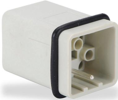
ZIPport male insert, connector housing size 3A, 12-pole, crimped contact, 10 amp, 600 VAC/VDC, poles numbered 1 to 12. For use with ZIPport multi-wire housings. Requires 10 amp male contacts ZP-MC-CC-M10A-xxx.
