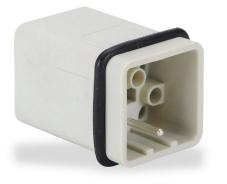
ZIPport male insert, connector housing size 3A, 12-pole, crimped contact, 10 amp, 600 VAC/VDC, poles numbered 1 to 12. For use with ZIPport multi-wire housings. Requires 10 amp male contacts ZP-MC-CC-M10A-xxx.
