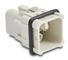
ZIPport male insert, connector housing size 3A, 7-pole, crimped contact, 10 amp, 600 VAC/VDC, poles numbered 1 to 7. For use with ZIPport multi-wire housings. Requires 10 amp male contacts ZP-MC-CC-M10A-xxx.
