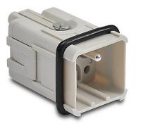
ZIPport male insert, connector housing size 3A, 5-pole, crimped contact, 16 amp, 600 VAC/VDC, poles numbered 1 to 5. For use with ZIPport multi-wire housings. Requires 16 amp male contacts ZP-MC-CC-M16A-xxx.
