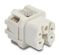
ZIPport female insert, connector housing size 3A, 4-pole, screw terminals, accepts wire size 20 - 14 AWG, 10 amp, 600 VAC/VDC, poles numbered 1 to 4. For use with ZIPport multi-wire housings.
