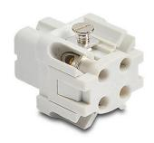
ZIPport female insert, connector housing size 3A, 3-pole, screw terminals, accepts wire size 20-14 AWG, 10 amp, 600 VAC/VDC, poles numbered 1 to 3. For use with ZIPport multi-wire housings.
