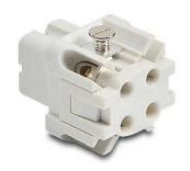
ZIPport female insert, connector housing size 3A, 3-pole, screw terminals, accepts wire size 20 - 14 AWG, 10 amp, 600 VAC/VDC, poles numbered 1 to 3. For use with ZIPport multi-wire housings.
