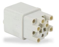
ZIPport female insert, connector housing size 3A, 12-pole, crimped contact, 10 amp, 600 VAC/VDC, poles numbered 1 to 12. For use with ZIPport multi-wire housings. Requires 10 amp female contacts ZP-MC-CC-F10A-xxx.
