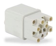
ZIPport female insert, connector housing size 3A, 12-pole, crimped contact, 10 amp, 600 VAC/VDC, poles numbered 1 to 12. For use with ZIPport multi-wire housings. Requires 10 amp female contacts ZP-MC-CC-F10A-xxx.
