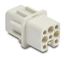
ZIPport female insert, connector housing size 3A, 7-pole, crimped contact, 10 amp, 600 VAC/VDC, poles numbered 1 to 7. For use with ZIPport multi-wire housings. Requires 10 amp female contacts ZP-MC-CC-F10A-xxx.
