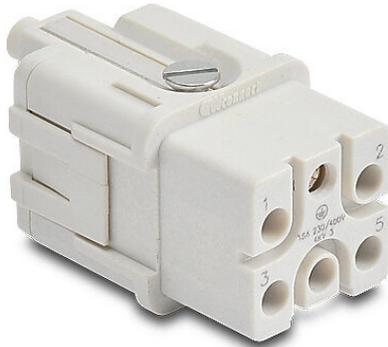
ZIPport female insert, connector housing size 3A, 5-pole, crimped contact, 16 amp, 600 VAC/VDC, poles numbered 1 to 5. For use with ZIPport multi-wire housings. Requires 16 amp female contacts ZP-MC-CC-F16A-xxx.
