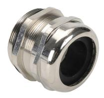
ZIPport cable gland, PG36 thread type, nickel-plated brass, accepts 19 to 36mm diameter cable, IP68. Package of 5.
