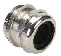
ZIPport cable gland, PG36 thread type, nickel-plated brass, accepts 19 to 36mm diameter cable, IP68. Package of 5.
