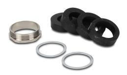
ZIPport cable gland, PG36 thread type, nickel-plated brass, accepts 19 to 36mm diameter cable, IP66. (4) elastomer compression seals included.
