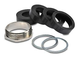
ZIPport cable gland, PG29 thread type, nickel-plated brass, accepts 17.5 to 26.5mm diameter cable, IP66. (4) elastomer compression seals included.
