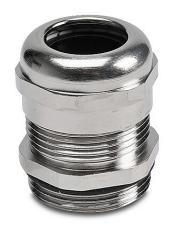
ZIPport cable gland, PG21 thread type, nickel-plated brass, accepts 11 to 18mm diameter cable, IP68. Package of 5.
