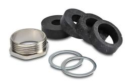
ZIPport cable gland, PG21 thread type, nickel-plated brass, accepts 9.5 to 18.5mm diameter cable, IP66. (4) elastomer compression seals included.
