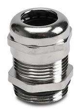
ZIPport cable gland, PG16 thread type, nickel-plated brass, accepts 8 to 14mm diameter cable, IP68. Package of 10.
