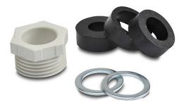
ZIPport cable gland, PG11 thread type, polyamide, light gray, accepts 7 to 12mm diameter cable, IP66. (3) elastomer compression seals included.
