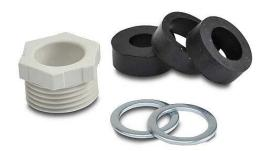
ZIPport cable gland, PG11 thread type, polyamide, light gray, accepts 7 to 12mm diameter cable, IP66. (3) elastomer compression seals included.
