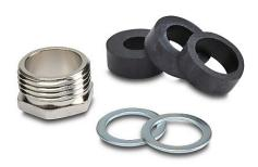
ZIPport cable gland, PG11 thread type, nickel-plated brass, accepts 7 to 12mm diameter cable, IP66. (3) elastomer compression seals included.
