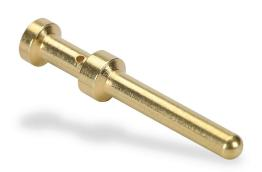
ZIPport crimp contact, male, 16 amp, accepts wire size 26-22 AWG, gold-plated copper alloy. Package of 100. For use with ZIPport multi-wire male inserts rated for 16 amps.
