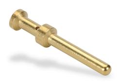
ZIPport crimp contact, male, 16 amp, accepts wire size 20 AWG, gold-plated copper alloy. Package of 100. For use with ZIPport multi-wire male inserts rated for 16 amps.
