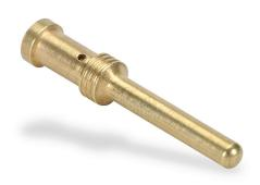
ZIPport crimp contact, male, 16 amp, accepts wire size 14 AWG, gold-plated copper alloy. Package of 100. For use with ZIPport multi-wire male inserts rated for 16 amps.
