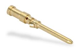
ZIPport crimp contact, male, 10 amp, accepts wire size 26-22 AWG, gold-plated copper alloy. Package of 100. For use with ZIPport multi-wire male inserts rated for 10 amps.
