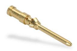
ZIPport crimp contact, male, 10 amp, accepts wire size 20 AWG, gold-plated copper alloy. Package of 100. For use with ZIPport multi-wire male inserts rated for 10 amps.
