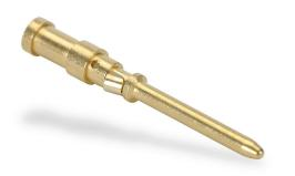
ZIPport crimp contact, male, 10 amp, accepts wire size 18 AWG, gold-plated copper alloy. Package of 100. For use with ZIPport multi-wire male inserts rated for 10 amps.
