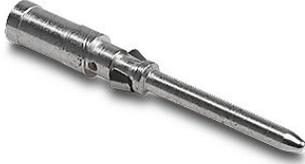
ZIPport crimp contact, male, 10 amp, accepts wire size 16 AWG, silver-plated copper alloy. Package of 100. For use with ZIPport multi-wire male inserts rated for 10 amps.
