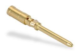
ZIPport crimp contact, male, 10 amp, accepts wire size 16 AWG, gold-plated copper alloy. Package of 100. For use with ZIPport multi-wire male inserts rated for 10 amps.
