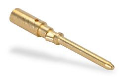
ZIPport crimp contact, male, 10 amp, accepts wire size 14 AWG, gold-plated copper alloy. Package of 100. For use with ZIPport multi-wire male inserts rated for 10 amps.
